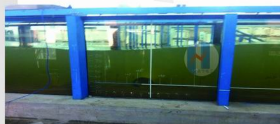
模拟海底暗涌造浪试验 Simulated submarine undercurrents and making wave test
